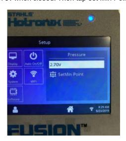
2. It may say Calibration Successful, but you can disregard and just tap Calibrate again. It will adjust to display a voltage on the screen in the 2.50v range approx.
