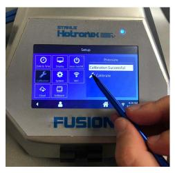
After setting the Min Point, lift the handle back up and increase the pressure knob clockwise again to set the max point. You want 3.0v to display when the press is closed. Then tap set Max Point.
