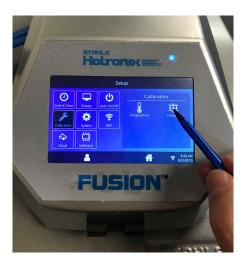
3. When you lock your press handle down the voltage number will change. You will need to manually adjust the pressure and lock the press down until it is set to around 2.70v when closed. Then tap set Min Point.
